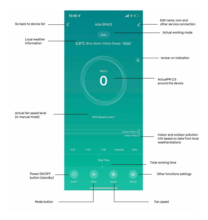
**8.** You can also use the application to control the individual functions of the purifier. Using the MODE button you can select the operating mode (Manual mode, Auto mode, Speed mode (maximum power), Sleep mode), use the SPEED button to control the fan speed. You can also set other functions - ionizer (Anion), child lock (Lock) and timer.
